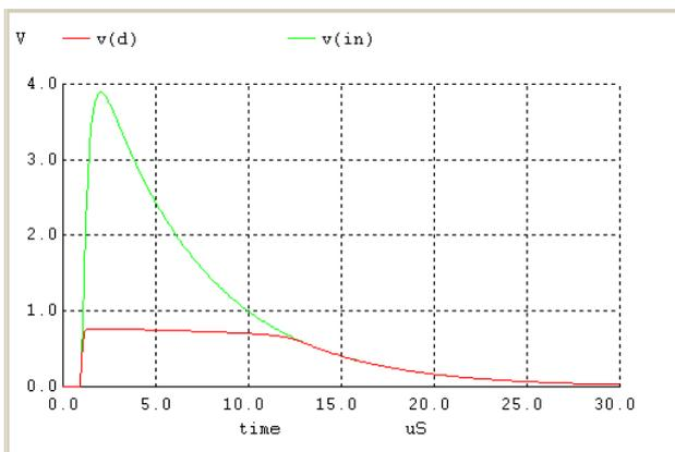
Fig. 2 Clipping a pulsed signal
