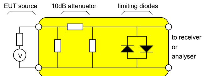
Fig. 1 Simplified limiter schematic
