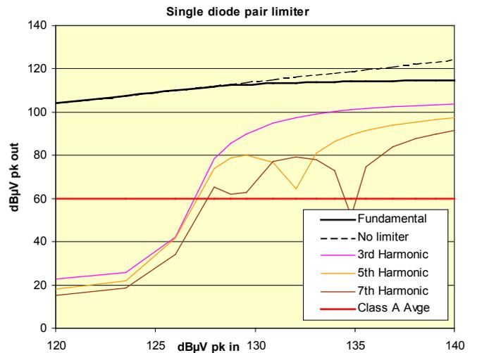
Figure 5 Harmonic output vs. input of the single pair limiter
