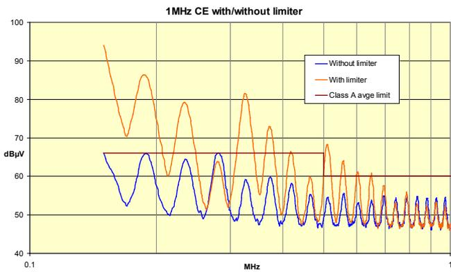
Fig 3 The example EUT from 150kHz to 1MHz, with and without a limiter in place
