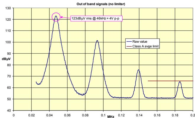
Fig. 4 The lower frequency fundamental and harmonics
