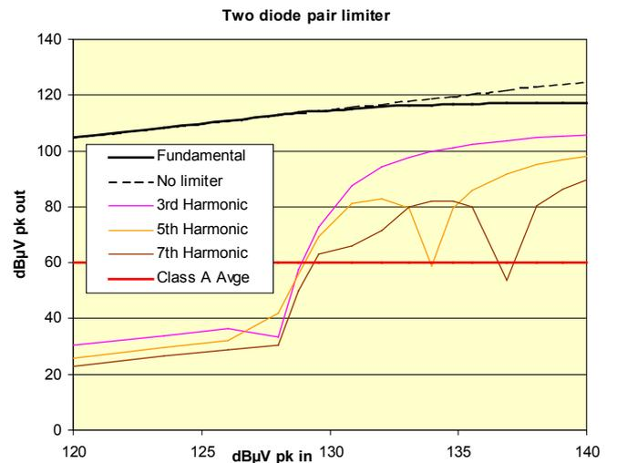
Figure 6 Harmonic output vs. input of the dual pair limiter
