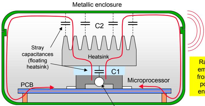
Circulating currents developed in enclosure via C1 and C2
