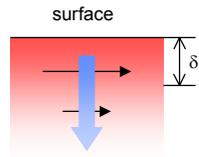
Current density drops 8.6dB for every  $\delta$  penetration: low values of  $\delta$  give good absorption
